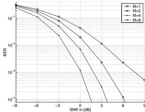
Fig. 6. BER of OFDM systems without CP applying antenna diversity.
