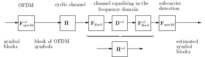
Fig. 3. OFDM system without guard period.
