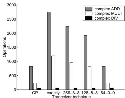
Fig. 5. Computational requirements of different transceiver techniques.
