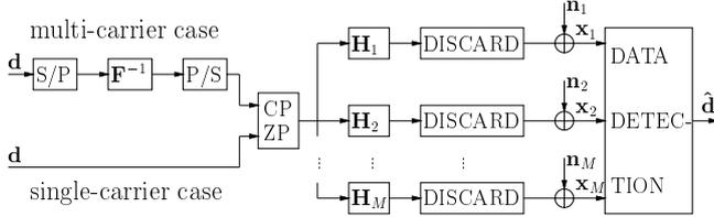
**Fig. 1.** Transmission system with multiple receiving antennas.
