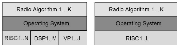
Figure 6 Heterogeneous and homogeneous multi-processor platform for Software Radio.
