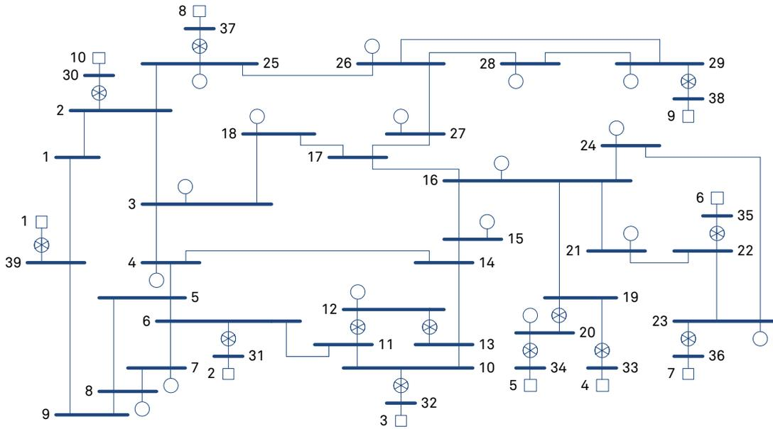
Figure 1: IEEE 39-bus New England Test System
