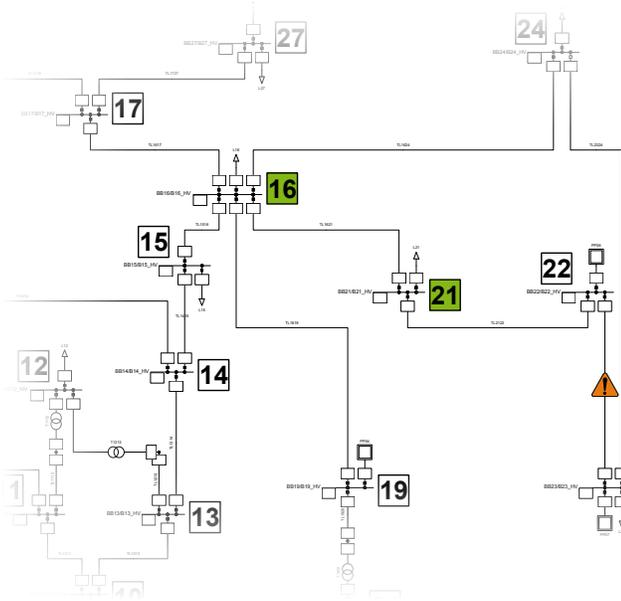
Figure 2: Cutout of the *New England Test System* (Fig. 1) as modeled in *PowerFactory*
